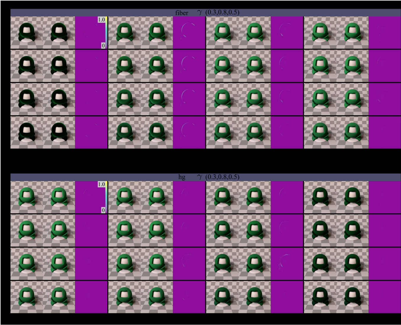
Fig. 1. Multiple scattering validation for a set of single-layer materials, over varying thickness and roughness. Monte Carlo simulation of multiple scattering is used as the ground truth. We find small differences from the ground truth.
